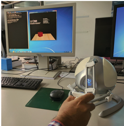
Fig. 2. An illustration of the hardware setup: user interacting with the virtual environment by a Falcon haptic device.
