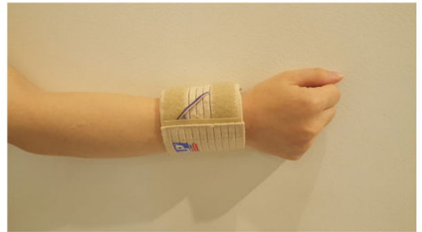
Fig. 14. The wristband device used in experiment 2 (Note that the vibrotactile motors are embedded in the wristband).
