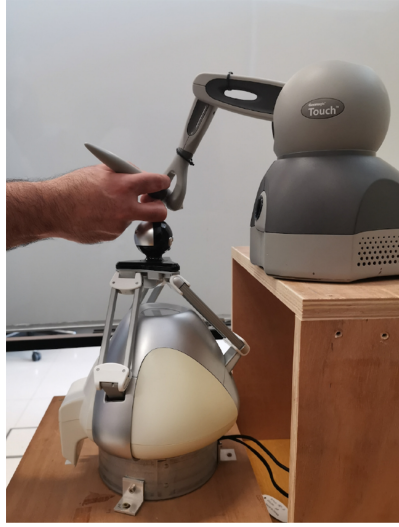
Fig. 5. Finger support system.
