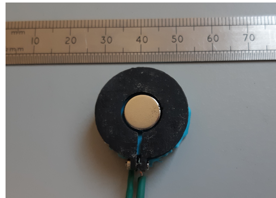
Fig. 2. A prototype of the vibrotactile actuator next to a ruler for scale
