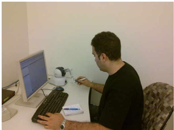
Fig. 2 Experimental setup where the user is manipulating the haptic device to write a particular letter on the writing pane
