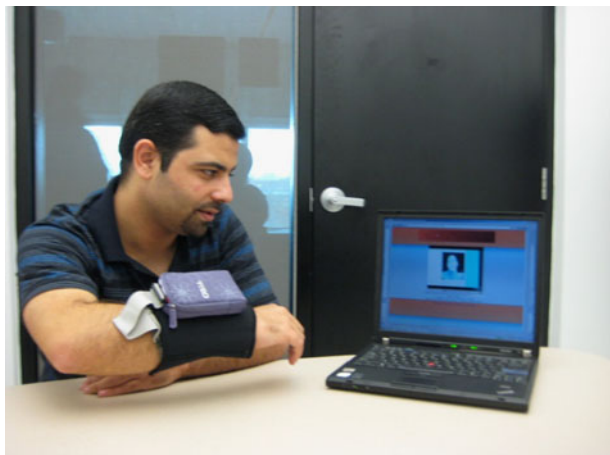
Fig. 6 Experimental setup where the user is watching a video and receiving synchronous tactile feedback via the arm bend device
