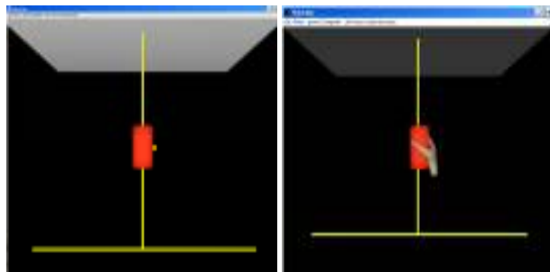
Figure 3. Snapshot of the application using OMNI (Single contact point with the VE) and CyberGrasp (multiple contact point with the VE)
