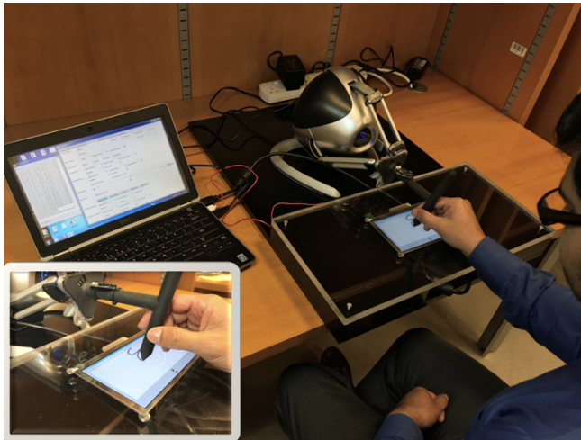
Fig. 1: Novint's Falcon™ haptic device used in experiments. The children grab the pencil-shaped end effector and the haptic device guides the participants' handwriting to know how to write the task letter or draw task shape.
