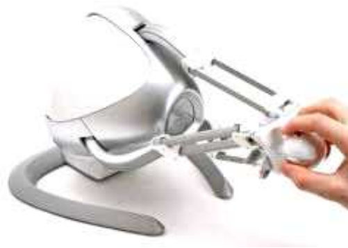
Fig. 4.20: The Novint Falcon device
