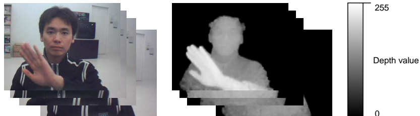
Fig. 6.4: A representation of a 2.5D video that has touchable geometry information and haptic surface
