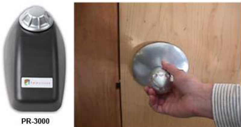
Fig. 4.12: Rotary controls from Immersion Corp. can be programmed with a wide variety of tactile sensations. (a) The PR-3000 Rotary Control with a Motor Actuator provides more sophisticated dynamic effects, such as springs and notches, (b) The “Aladdin” is a half-door with a fully functional knob, latch control, door angle sensing, and an auditory display
