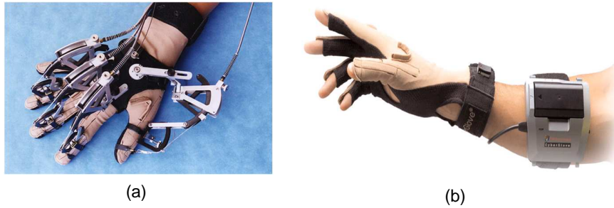
Fig. 4.16: (a) The CyberGrasp force feedback system, (b) The CyberGlove interface
