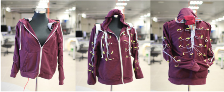
Fig. 2. Haptic jacket design.
