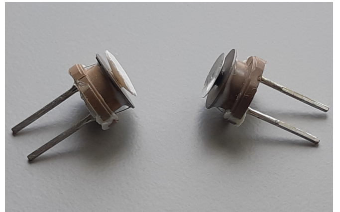
Fig. 5. Left: Modified transducer, Right: original transducer
