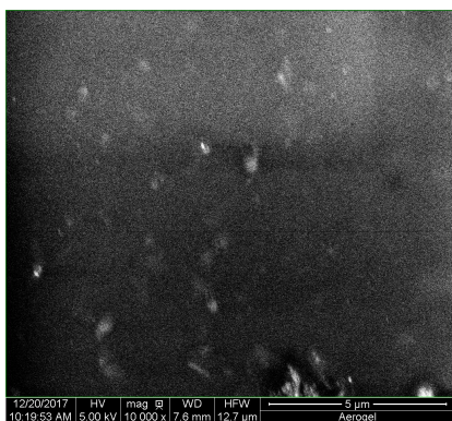
Fig. 3. Airloy structure under scanning electron microscopy
