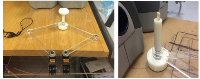
Fig. 6. (left) 2 DoF parallel robotic device for finger rest, (right) Finger rest end effector with a tooth model attached.
