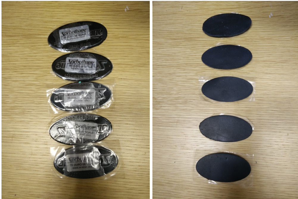
(a) Labeled side of the Sorbothane samples. (b) Backside of the Sorbothane samples. This side was subjected to the ultrasonic radiation.
